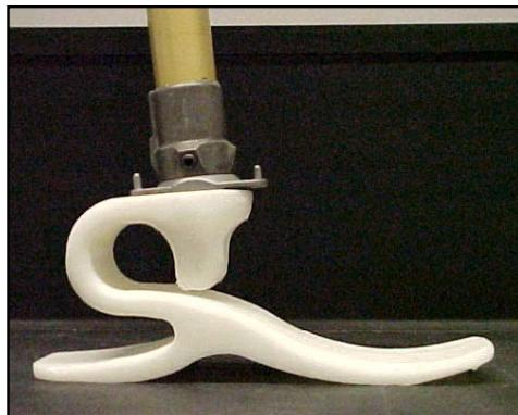
**Figure 1.** Niagara Foot prosthetic component. The one-piece component facilitates plantarflexion on heel strike and significant energy return on toe-off. The component is compatible with existing prosthetic systems such as the Otto Bock units shown.
