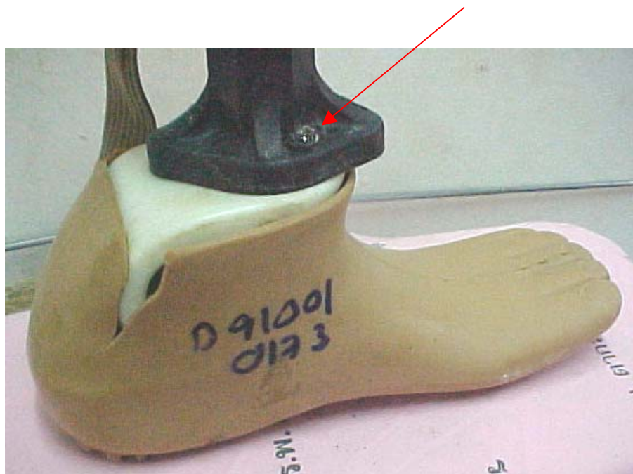
Figure 9: Cover tear. Typical pattern of tear observed in covers. Note counter-rotation screw at the arrow.
