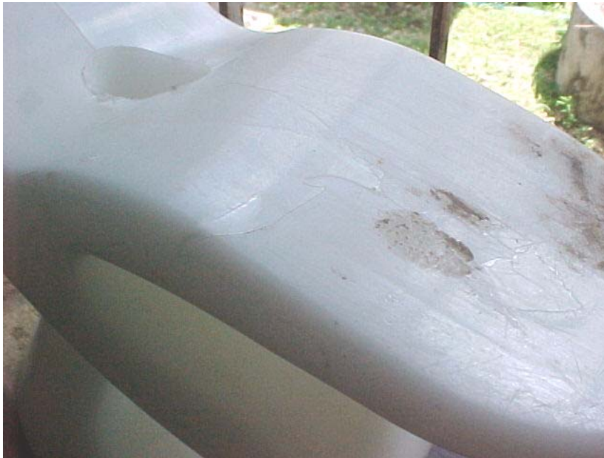
Figure 6: Non-structural surface scratching. These effects are likely due to third body wear from sand or debris trapped in the cover.
