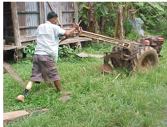
Figure 16: Farmer. The primary device used is a motorized “tractor”. (a, top) The trailer can be removed or attached by a pin connection. (b, bottom) When plowing, the operator must exert an upward reaction force while walking on uneven ground.
