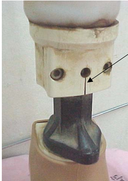
Figure 12: Socket-Pylon interface cracking. A vertical crack is apparent at the connection.
