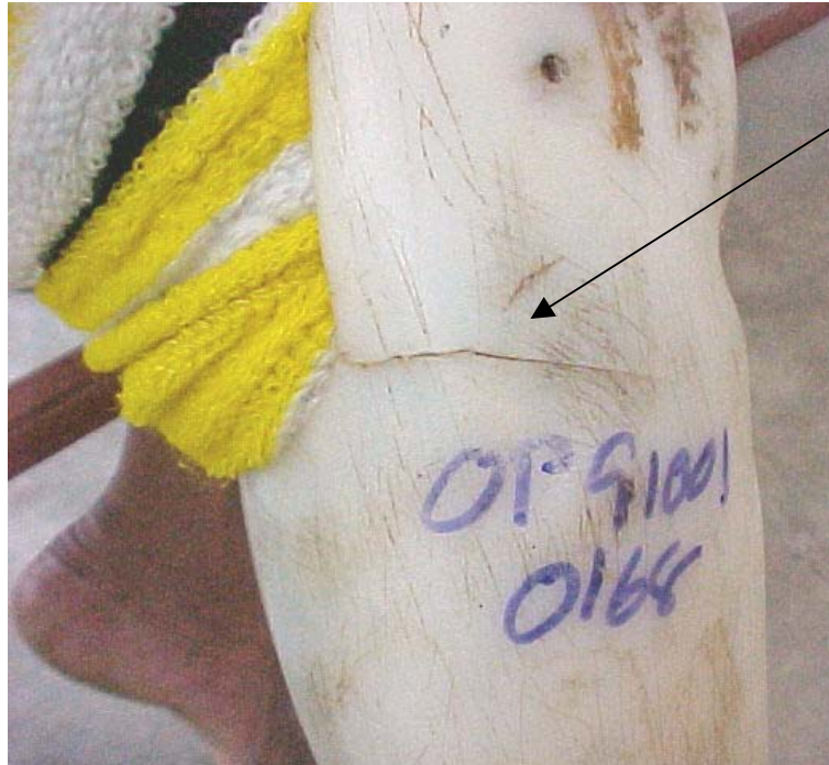
Figure 10: Socket cracking. Two sockets exhibited cracking in the proximal region near the epicondyles. In both cases the crack progressed anteriorly.
